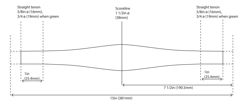
Turn oversive at 15in - Final length, and position of scoreline, are determined during fitting.
