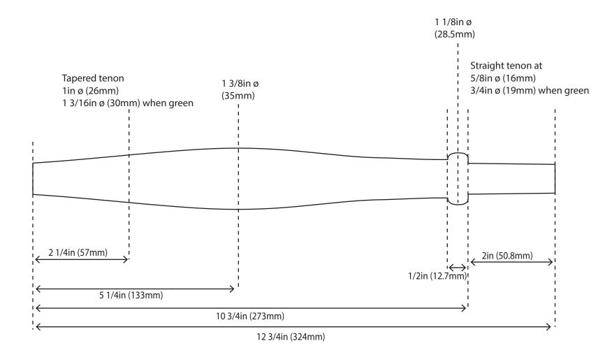
\*Turn all components oversize whilst green. Final sizing is done once components have finished drying.
